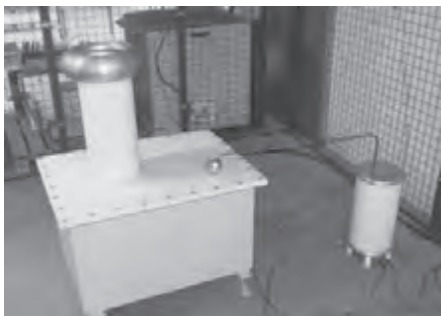
Partial discharge equipment available up to 100kV
