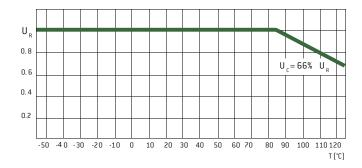
For the types which can be used up to  $200^{\circ}$ C, the voltage must be derated between +85°C and +200°C according to the following curve.
