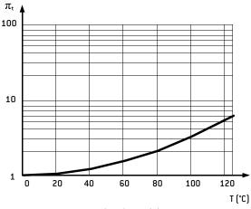
Formula:  $\pi_t = \exp(1,8.(t/tm)^2)$ with: t = using temperaturetm = maximum temperature
